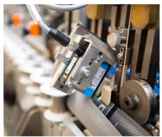
NEOSeam allows tube producers to re-purpose the «side trim», the laminate material which is normally cut off the printed material and then thrown away. The side-trim is used by NEOSeam to build-up the tube's sideseam, allowing the production of tubes which do not show any «white line» at the side seam area even after multiple uses.
